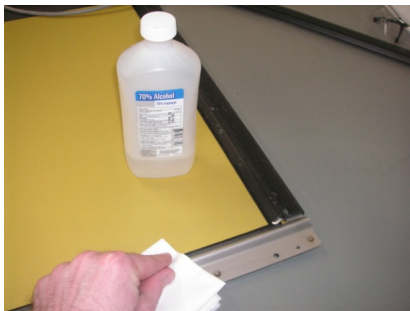
Figure 13: Cleaning Edge Protector
