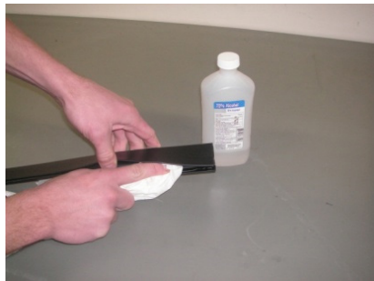
Figure 20: Cleaning Vinyl Edge Cover
