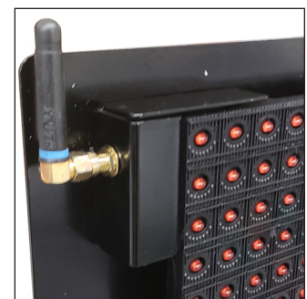
Figure 3: Antenna Bracket Correctly Installed
