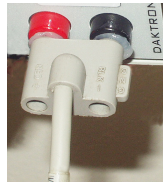
Figure 10: Insert GND Side to Black Female Jack
