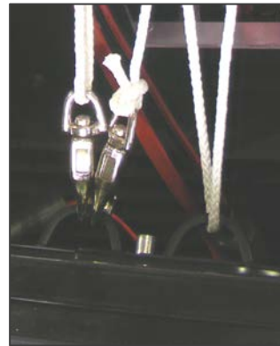
Figure 15: Safety Lanyard Attached to Module Lanyard Attachment Rings
