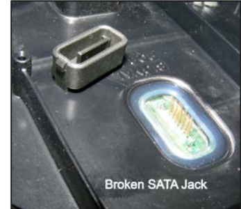
Figure 3: Broken SATA Jack
