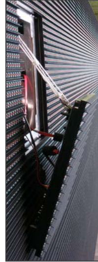
Figure 17: Module Safety Lanyard Prevents Module from Falling
