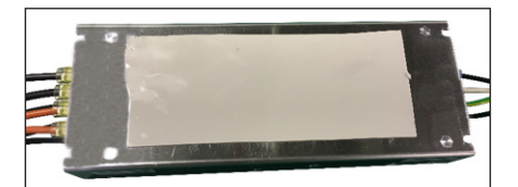
Figure 44: Thermal Pad on Power Supply
